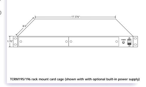
The TCRM195 and TCRM196 Universal Rack Mount Card Cages hold up to two single multiplexer or modem-type cards, or one double-mux or double-modem type card. In general the TCRM195 is used for multiplexers and the TCRM196 for modems.
