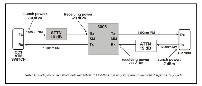
Figure 5. In-line Attenuator Placement Diagram
