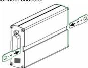
3. Attach the adapter to the surface with two screws.
