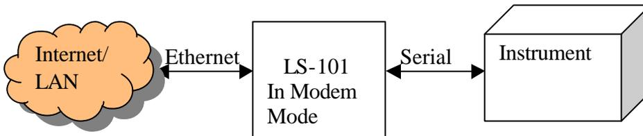
Fig2. Modem mode of operation.
