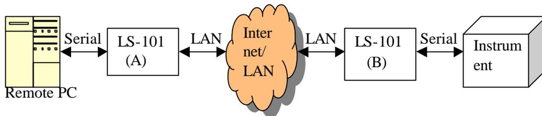
Fig. 2. Internet/LAN enable the serial device (Server running serial software)
