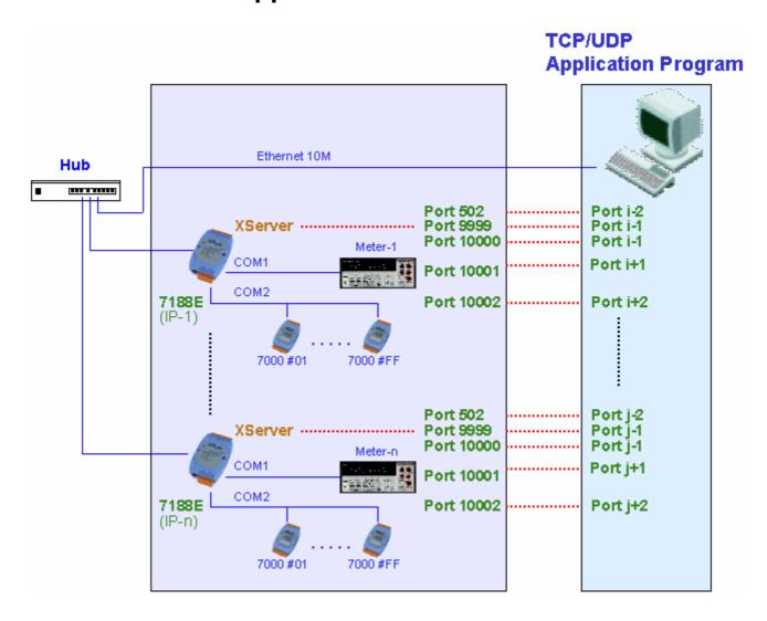
The Xserver is a powerful program designed for Ethernet I/O applications. It supplies the 7188E with a range of flexible options. Users can modify the Xserver to control all of the 7188E's hardware: COM ports, I/O expansion boards, a 7 Seg LED, or other relevant products.
