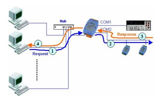
Condition 2: No clients send any request to Xserver to access devices. The Xserver doesn't echo data from devices to any client.
