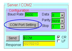
Step 6: Send "\$03M" to read 7000 module's ID which is connected to 7188E3's COM3.
