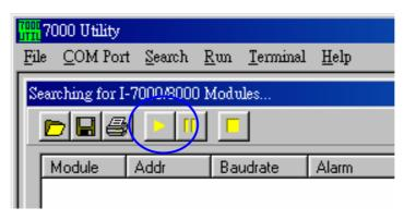
Step 5: If the VxComm Driver works well, the 7000 Utility can search the module(s) connected to the 7188E/8000E's COM1.
