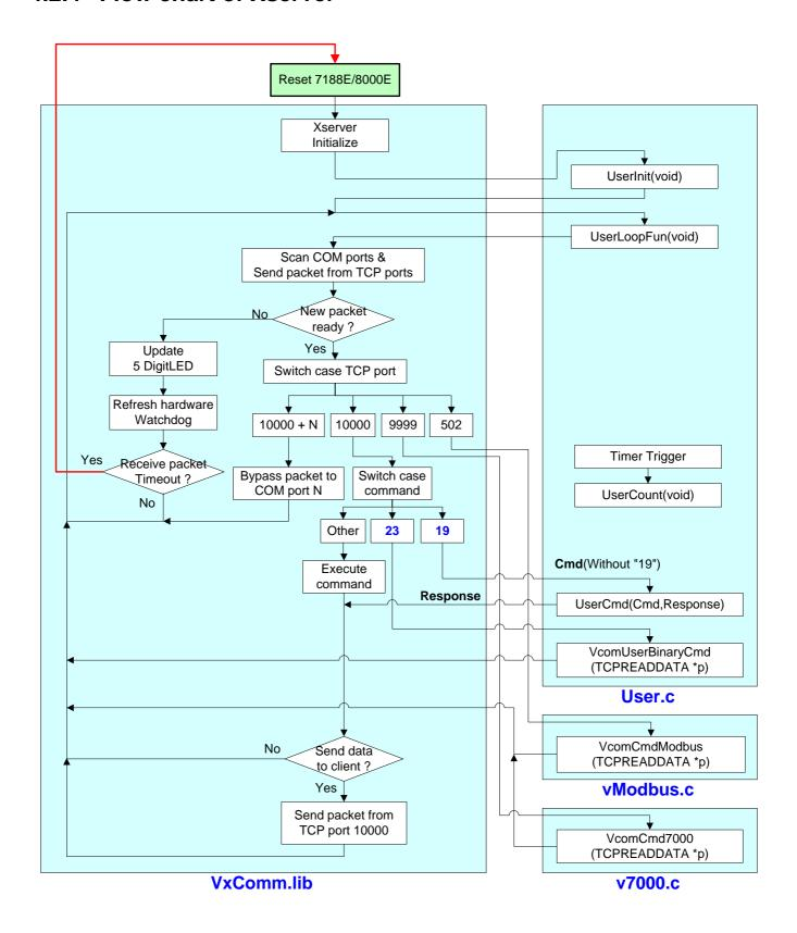
It is very difficult to develop an embedded controller program with Ethernet/Internet communication. But by using the Xserver, users can do that quickly and easily. Users need only modify 7 functions in User.c, vModbus and v7000.c. Users build their own code in the 7 functions to make the Xserver work as they desire. The features of the 7 functions are listed below:
