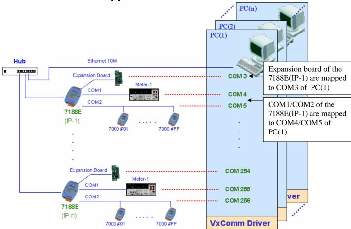
To use the Virtual COM application, first install the VxComm Driver. After installation, the VxComm Utility can map any 7188E's remote COM port. These virtualized COM ports can be used by the PC to control devices directly, just as you would use COM1 (real COM port) to control devices. When using the Virtual COM application, one PC can use a maximum of 256 COM ports. Users need not worry about network connections. The VxComm Driver will handle all Ethernet/Internet connections.
