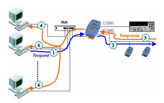
Condition 2: No clients send a request to Xserver to access devices. The Xserver echoes data from devices to every client which are connected to the 7188E/8000E.
