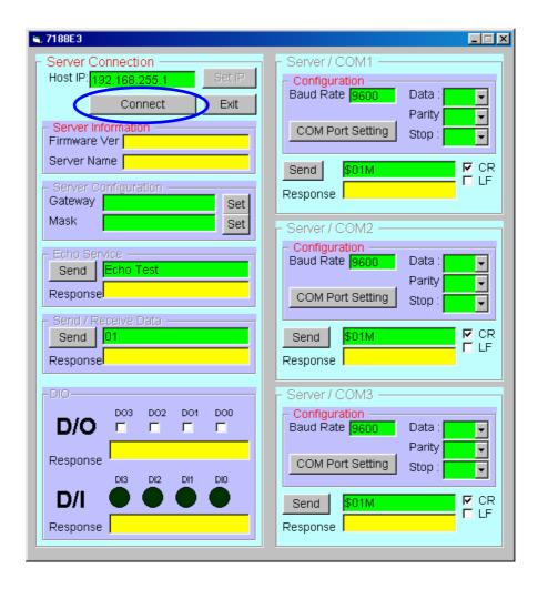
Step2: Press "Connect" button, and then the program will readout relative information concerning the 7188E3 and start scanning the DI of the 7188E3.
