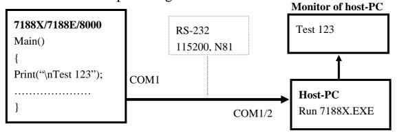
Keys-in test data from keyboard of host-PC
