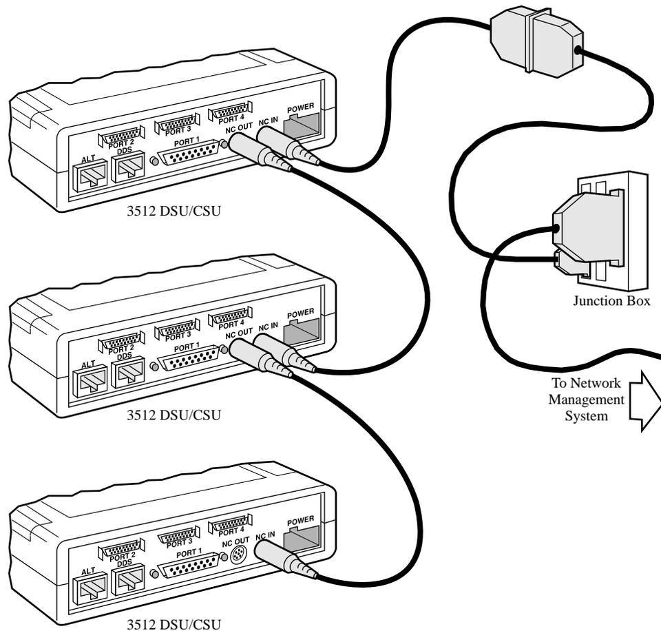
**Figure 2-6. Multiple Devices in a Daisy Chain Connection to NMS**
