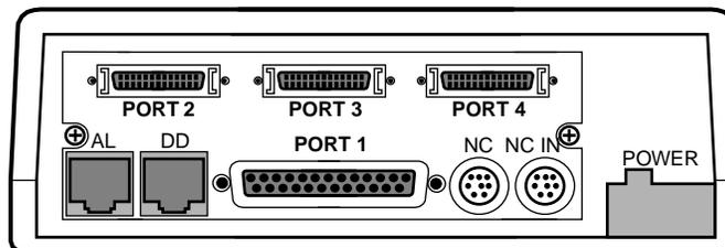
*Four -Port 3512 Rear Panel (Standalone)- Maximum Four DTE Connections*
