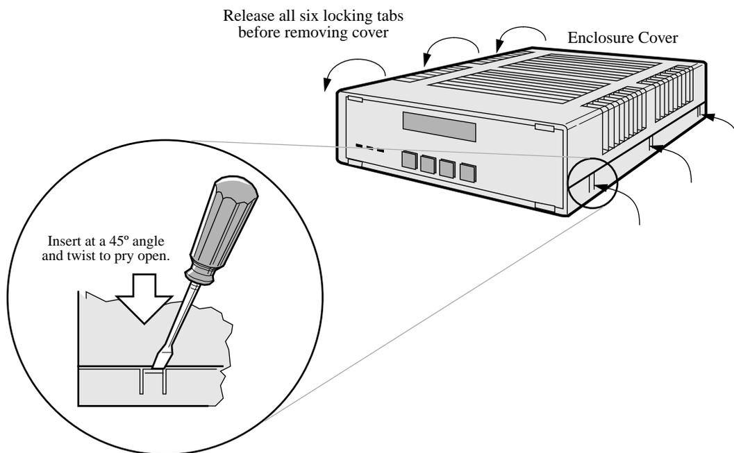
**Figure 2-7. Removing the 3512 Enclosure Cover**
