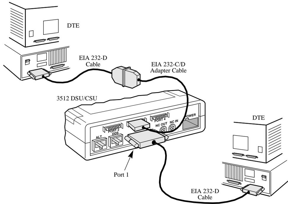
**Figure 2-4. 3512 Connection to DTEs**
