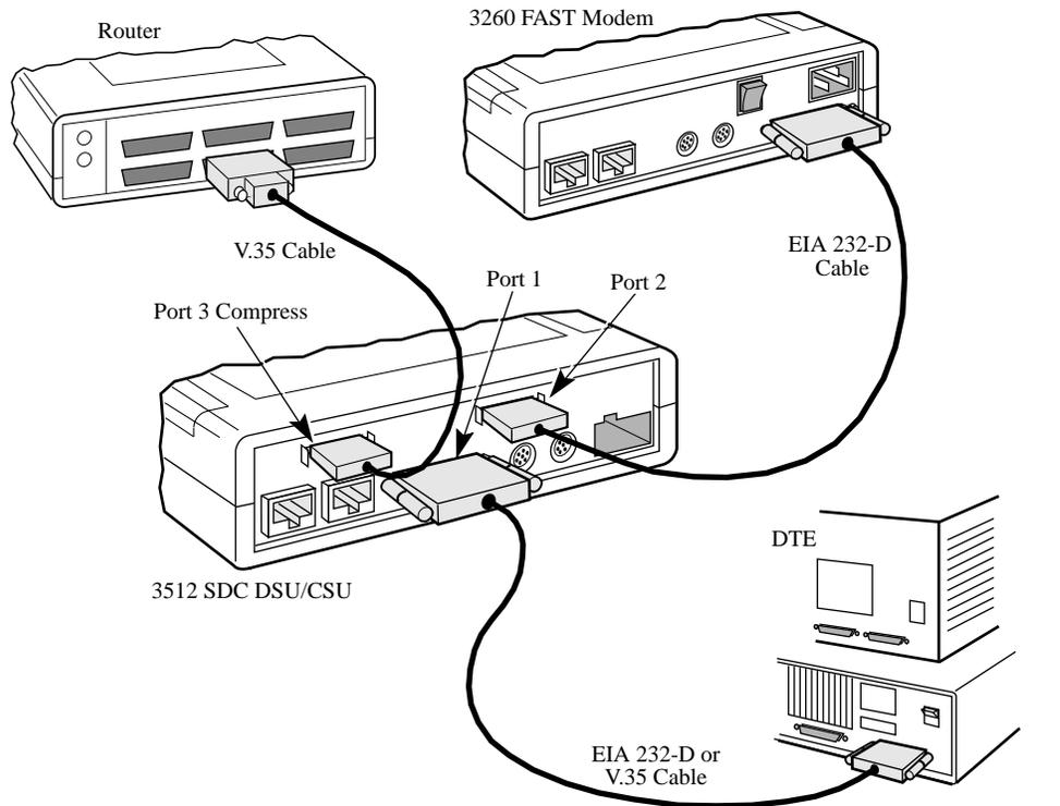
**Figure 2-5. 3512 SDC Connection to DTEs**
