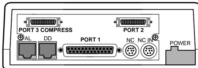
*Three-Port 3512 SDC Rear Panel (Standalone)- Maximum Three DTE Connections*
