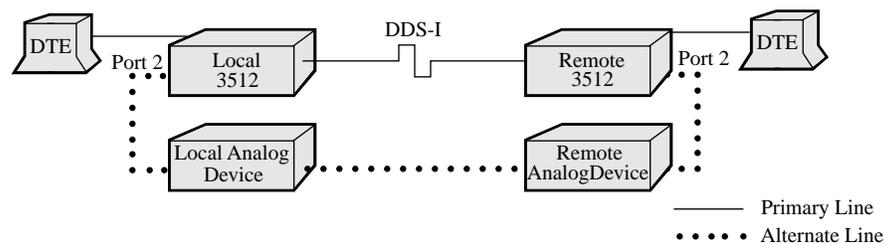
**Figure 2-3. Cabling for External Restoral**
