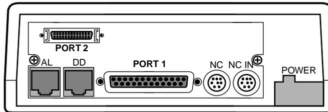
*Two-Port 3512 Rear Panel (Standalone)- Maximum Two DTE Connections*
