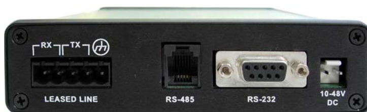
Figure 2-2. Back View of IG192HFP Modem
