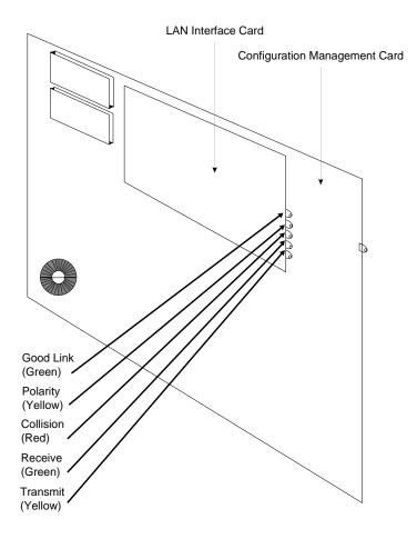
Figure 5-1 Piggyback LEDs for Debugging
